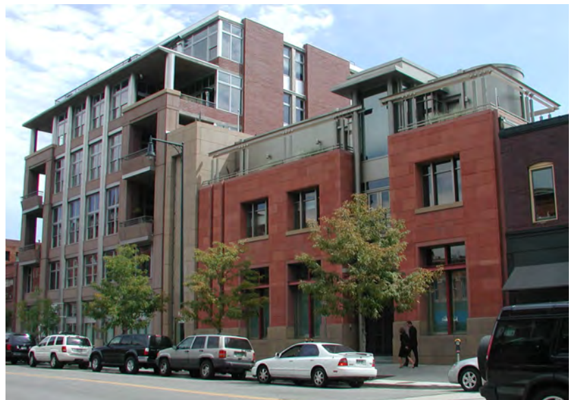
Fig. B.1.S1.b: Articulated wall planes break down building massing and frame the street.
