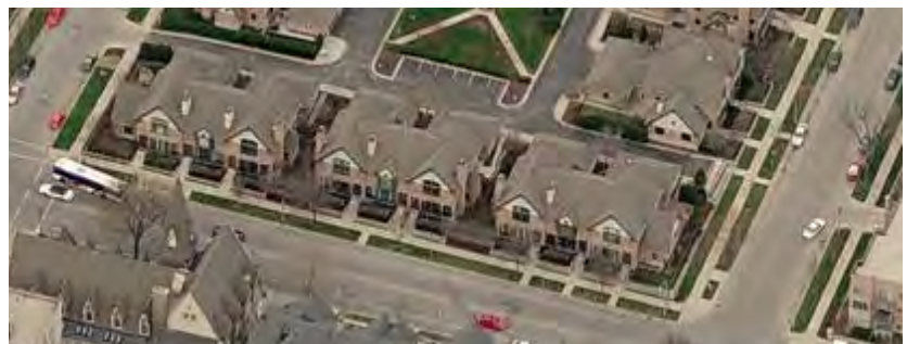
Fig. A.4.S2: Parking area is located behind multifamily buildings and accessed from a secondary frontage.
