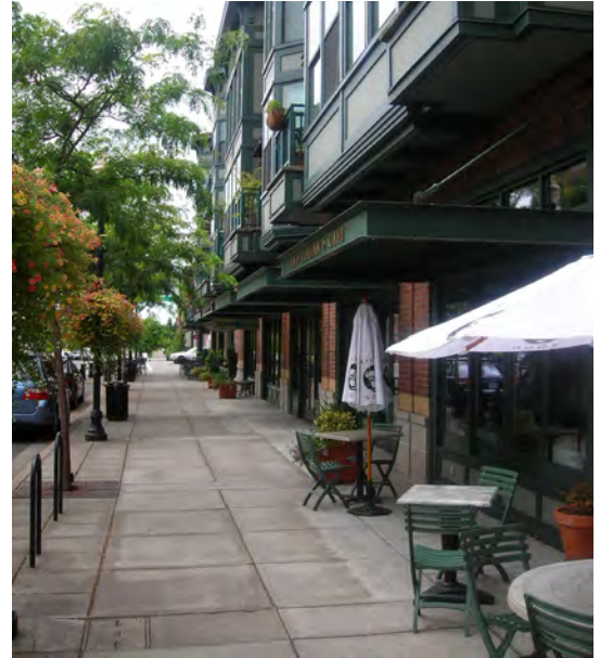
Fig. D.1 Wide sidewalks with active uses and tree wells in amenity zone.
