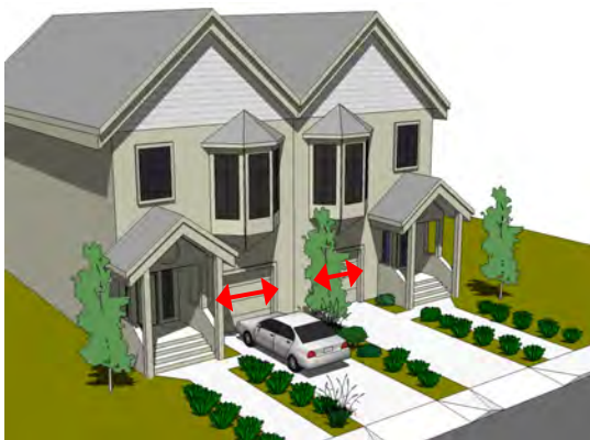
Fig. A.4.S13: Garage opening widths are less than 50 percent of the facade width of the unit they serve.
