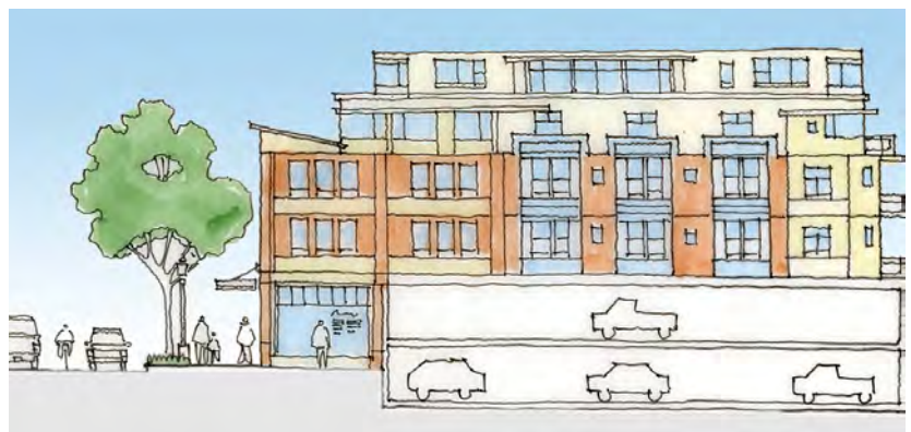
Fig. A.4.S4.b: Active street-level use serves as a liner space for a parking structure.
