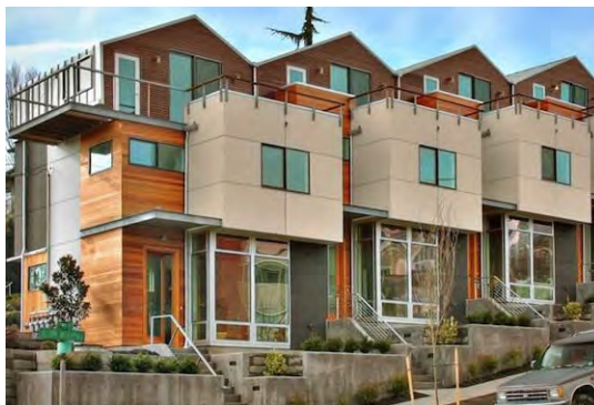
Fig. B.4.S15.a: Townhouses with gable roofs, facade offsets, cantilevered building masses, and multiple facade materials.
