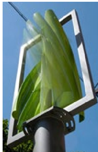
Small-scale, vertical-type wind turbine mounted on a pole.
